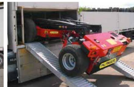
**ON TOP - DRIVEN ONTO LOAD PLATFORM
